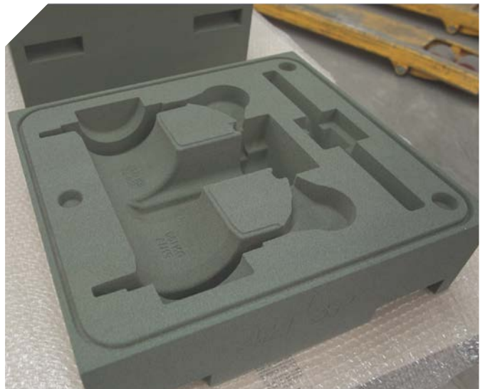
3D printed block assembling
